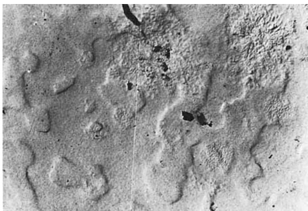
Fig. 2. Transmission electron micrograph of the two-stage replica annealing in argon atmosphere at 130^{\circ}\text{C} .
